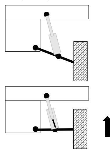
Because of the movement of the chassis on its suspension a vehicle will behave differently when accelerating or braking or turning. When accelerating a vehicle will lift the weight off the front wheels, when braking it will put more weight on the front wheels and when turning it will put more weight on the outside wheels. When this happens the amount of grip that the wheels have on the road is changed, more weight gives a vehicle more grip and less weight takes grip away.
