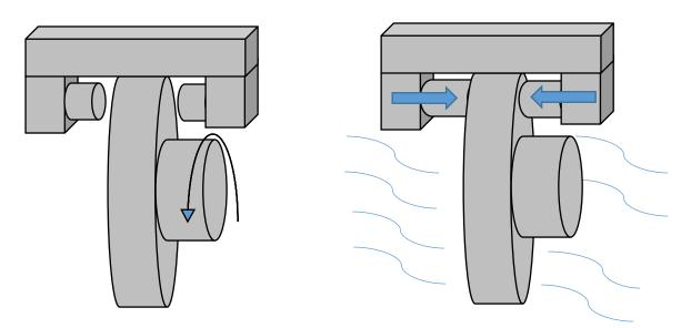
Because hydraulic systems have a tendency to loose pressure over long periods of handbrakes are usually mechanical and not hydraulic.
