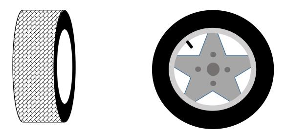
The height and flex of a tyre allows the tyre to act a bit like suspension absorbing bumps in the road, it also allows the tyre to bend to the shape of the ground giving it more grip.
